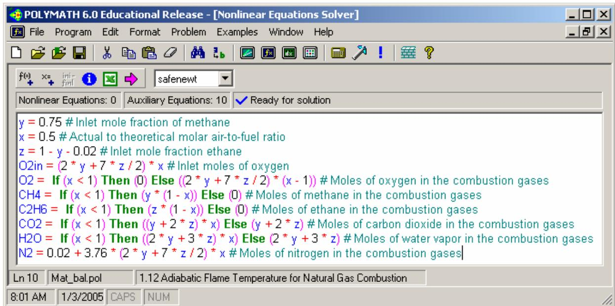
Figure 9. Polymath Program for Essential Material Balance Equations
