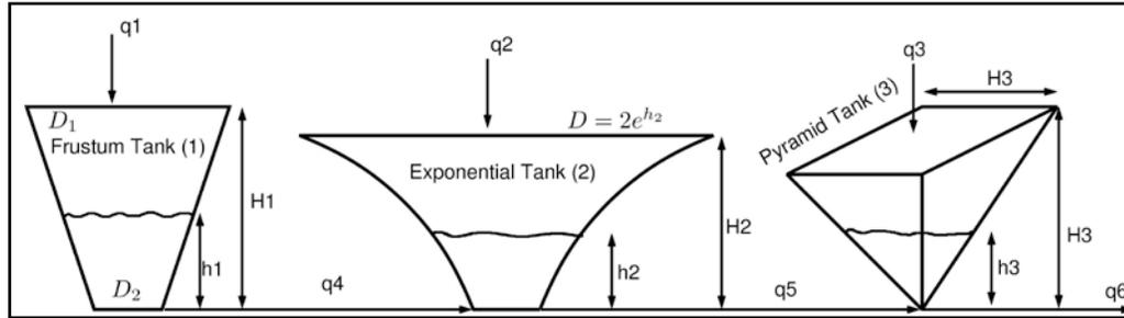
Figure 1. A Train of three interactive tanks.<sup>[4]</sup>
